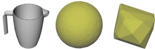
Fig. 16. Two 3D visualizations of the 6D object wrench space. The visualization in the middle shows the projection in force space and the projection in torque space is shown on the right. The shown OWS subspaces were built by setting the torque respectively the force to zero.
